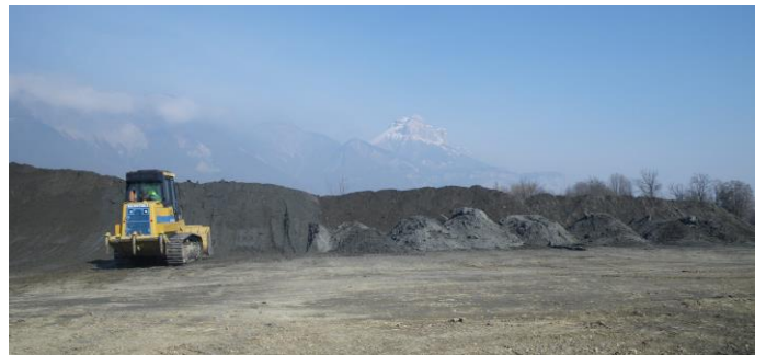
Figure 3. Silty gravels extracted from the Isere river.
